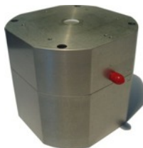
Integrating sphere - 80 mm diameter
