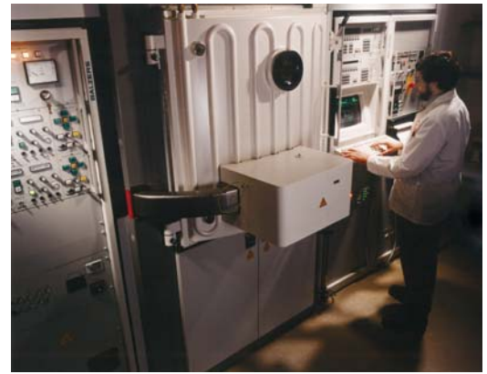
Newport's Stabilife Reactive Ion Plating Deposition System
